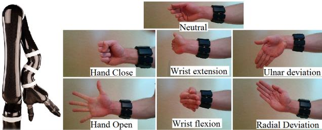
Fig. 1. The 7 gestures considered in this work. The Myo armband (right) is connected through bluetooth to the laptop. The computer, after data analysis, transfer the command to JACO (left) in real-time via a USB connection.
